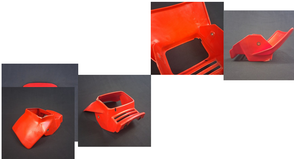
Front headlight fairing from a 1986 Honda XL250R
